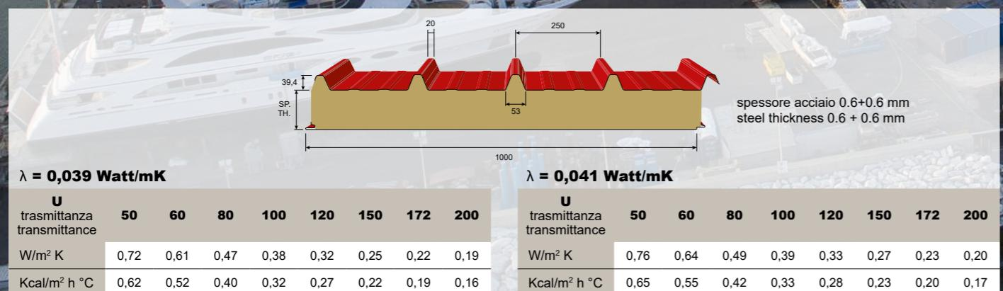
A RICHIESTA CON DENSITÀ DA 120 a 150 kg/m<sup>3</sup>. DENSITY FROM 120 to 150 kg/m<sup>3</sup> ON REQUEST
